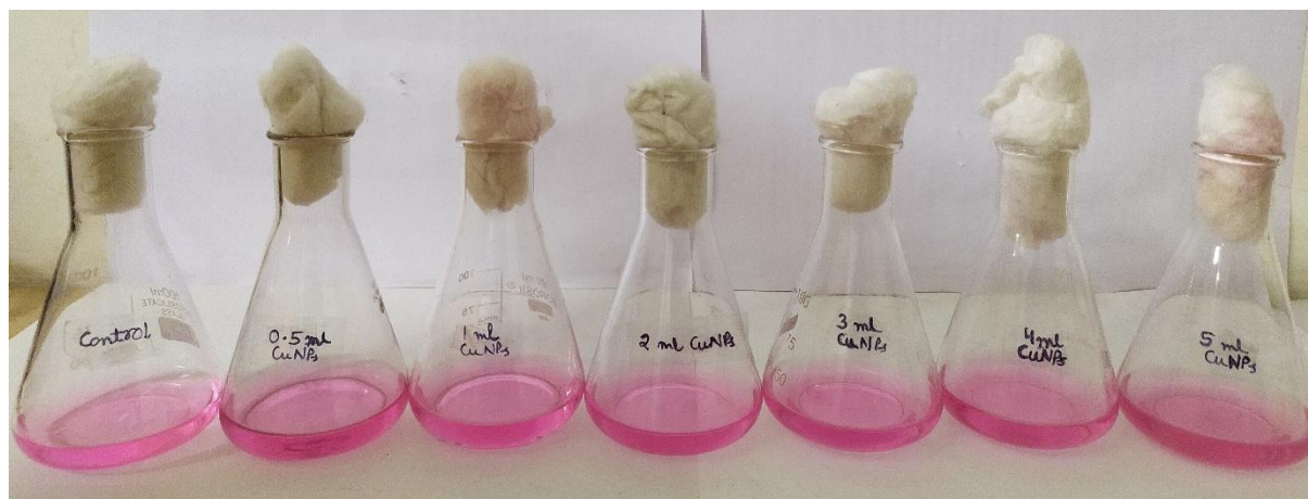
Figure 7. Same set of flasks as Figure 5, after 24 hours (without sunlight) of incubation at 37°C. A reduction is again observed in pink colour intensity with respect to Figure 6 with the increasing volumes of CuO nanoparticles, indicating dose-dependent degradation of the dye even without sunlight. The control flask remains unchanged, which confirms that the observed decolourization is due to CuO nanoparticles.
