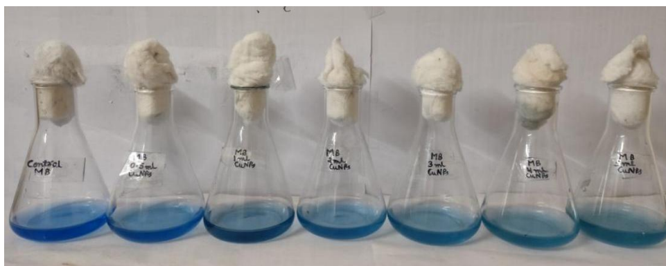
Figure 11: The same set of flasks as Figure 10, was kept in sunlight for up to 7 hours. A gradual reduction in Methylene Blue colour intensity is observed with the increasing volumes of CuO nanoparticles, indicating dose-dependent degradation of the dye.
