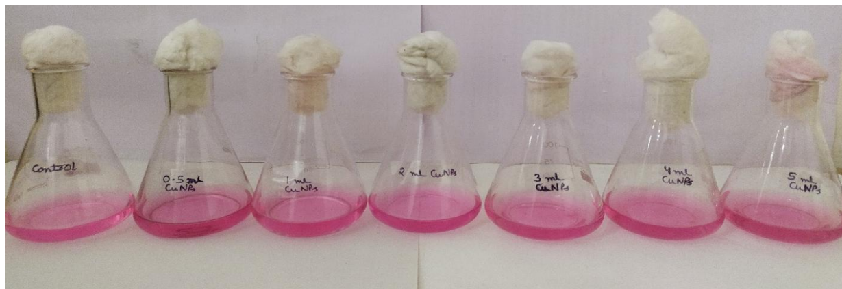
Figure 6. The same set of flasks as Figure 5, when kept in sunlight for up to 7 hours. A progressive reduction in pink colour intensity is observed with the increasing volumes of CuO nanoparticles, indicating dose-dependent degradation of the dye. The control flask remains unchanged, which confirms that the observed decolourization is due to the photocatalytic activity of CuO nanoparticles.
