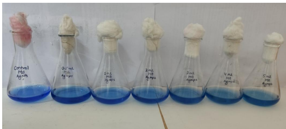
Figure 11: The same set of flasks as Figure 10, was kept in sunlight for up to 7 hours. A gradual reduction in Methylene Blue colour intensity is observed with the increasing volumes of CuO nanoparticles, indicating dose-dependent degradation of the dye.
