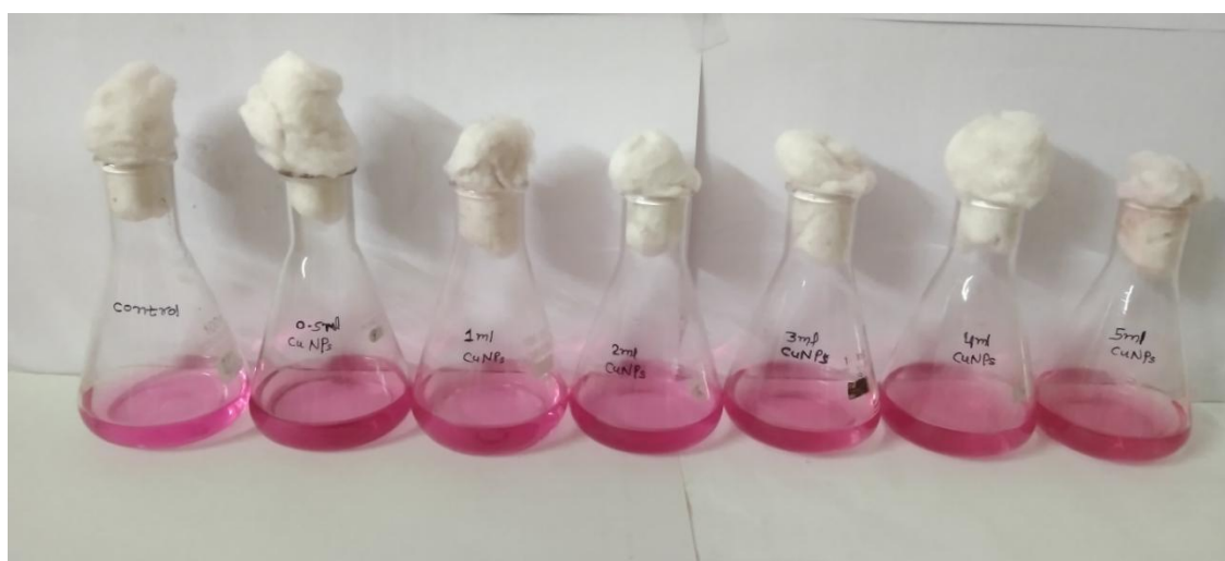
Figure 5. Erlenmeyer flasks containing 50 ppm Reactive Red dye solution immediately after the addition of varying volumes of biologically synthesized CuO nanoparticles (0.5 ml to 5 ml). The first flask is without nanoparticles. All flasks appear uniformly pink, indicating that no immediate decolourization has taken place at the onset of the reaction.
